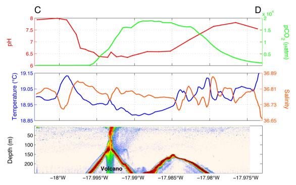
Figure 5 | Surface measurements of pH, pCO<sub>2</sub>, temperature and salinity along a transect across the volcano still show significant variations five months after the beginning of the eruptive process. Bottom panel shows an echogram from a 70 kHz echo sounder.
